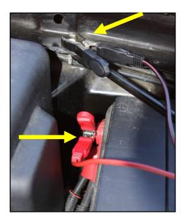
> Connect red clip to 12V-DC power.> Connect black clip to chassis ground.
