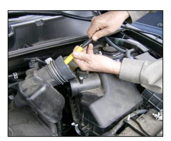
> Use cone to access intake system and connect smoke supply hose to cone.
