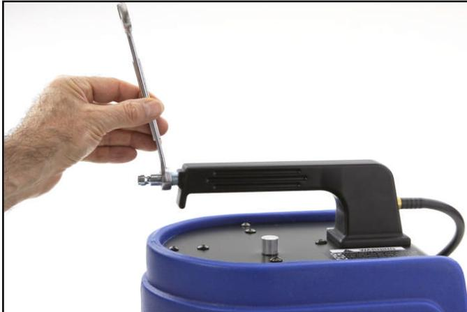
> If not supplied; install correct air fitting onto the Leakfinder®.
