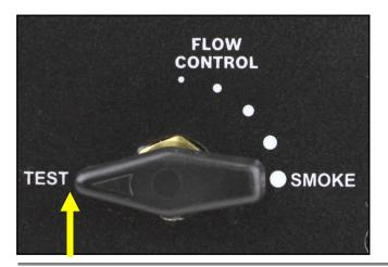
TEST: Delivers non-smoke air and the most accurate flow meter reading. This setting is for determining if a leak exists and how large it is.
