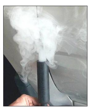
Smoke distrubance pinpoints the leak
