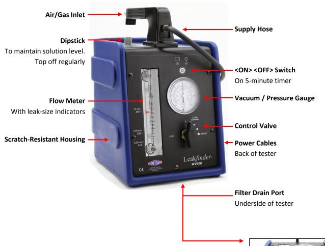
**Water Separator / Filter** (inside tester) with drain port at underside of tester; keeps tester and vehicle clean by automatically draining water and contaminants from workshop air compressor. It is normal to occasionally see drainage of fluid from this port. Excessive drainage indicates your air compressor requires draining and/or a filter system.
